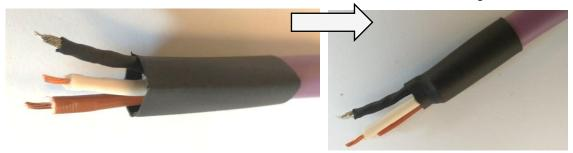
4. Solder the wires to the connector according to wiring diagram or instructions. Select the appropriate strain relief (other connector types might have different strain relief type than the one shown):
