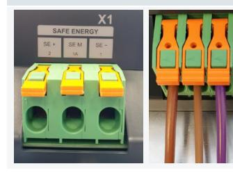
Connect the battery or Ultra Cap wires to the IMD X1 SAFE ENERGY connectors according to the wiring diagram and the instructions in section <u>5.2.1</u> on page <u>28</u>.
