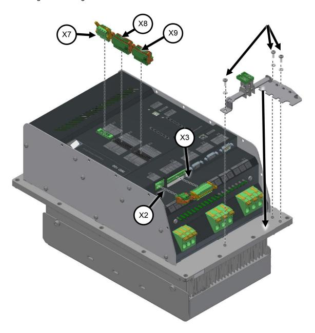
The shielding clamp is not mounted yet.
