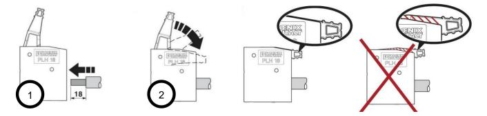
To take the wires out: Lift the handle and pull out the wire.
