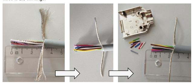
2. Strip approximately 3 mm insulation from the wires and solder the wires to the connector according to wiring diagram or instructions. Thread the shield's pigtails through the holes in the strain relief and roll them around the strain relief (other connector types might have different strain relief than the one shown):
