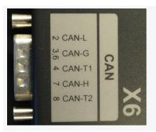
Mount a 9 pole D-sub female connector on the CAN communication cable according to the wiring diagram and the instructions in section <u>5.2.3</u> on page <u>30</u>.
