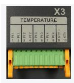
If applicable connect the sensors wires to the IMD X3 TEMPERATURE connectors according to the wiring diagram and the instructions in section <u>5.2.2</u> on page <u>28</u>.
