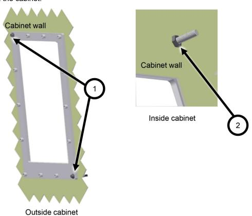
2. Mount the IMD on the two screws and fasten with nuts (Pos. 1). Ensure that all mounting holes in the heat sink are aligned with the holes in the cabinet (illustration of type C, applies also to type B).
