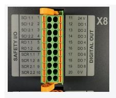
Mount the female FK-MCP 1.5 connector on X8 SAFETY I/O and DIGITAL OUT, and connect the wires according to the wiring diagram and the instructions in section <u>5.2.2</u> on page <u>28</u>.
