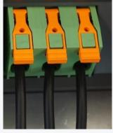
Connect the Mains wires to the IMD X1 MAINS connectors according to the wiring diagram and the instructions in section <u>5.2.1</u> on page <u>28</u>.
