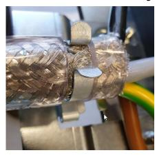
2. Fasten the cable with cable ties on both sides of the shielding clamp:
