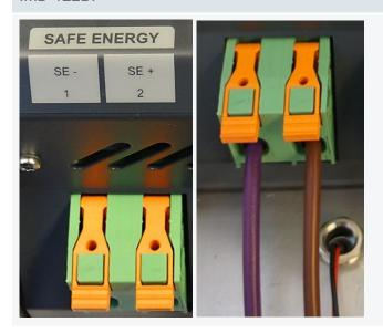
Connect the battery or Ultra Cap wires to the IMD X1 SAFE ENERGY connectors according to the wiring diagram and the instructions in section <u>5.2.1</u> on page <u>28</u>.
