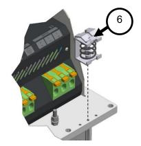
Figure 7 Mounting the shielding clamp directly on the heat sink
