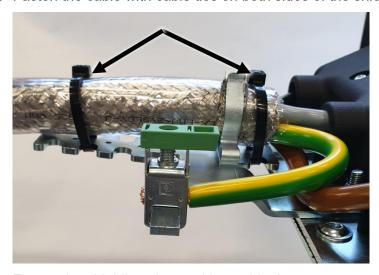
3. Fasten the shielding clamp with a cable tie:
