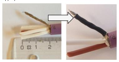
2. Strip approximately 3 mm insulation from the wires. Put 20 mm of appropriate size shrink tube around the cable. Ensure that the shield is covered. Shrink it with a heat gun:
