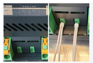
Connect the resistor's wires to the IMD X1 R-BALLAST connectors according to the wiring diagram and the instructions in section <u>5.2.3</u> on page <u>30</u>.
