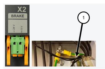
Connect the brake wires to the IMD X2 BRAKE connectors according to the wiring diagram and the instructions in section  $\underline{5.2.2}$  on page  $\underline{28}$ .
