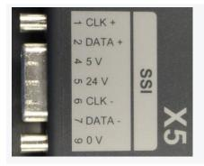
Mount a 9 pole D-sub male connector on the SSI cable according to the wiring diagram and the instructions in section <u>5.2.3</u> on page <u>30</u>.
