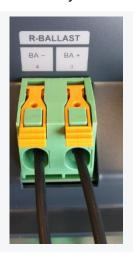
Connect the resistor's wires to the IMD X1 R-BALLAST connectors according to the wiring diagram and the instructions in section <u>5.2.1</u> on page <u>28</u>.
