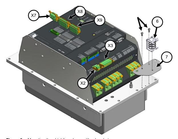
Figure 6 Mounting the shielding clamp with a bracket
