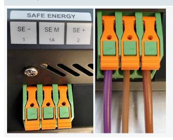
Connect the battery or Ultra Cap wires to the IMD X1 SAFE ENERGY connectors according to the wiring diagram and the instructions in section <u>5.2.1</u> on page <u>28</u>.
