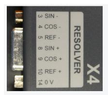
Mount a 15 pole D-sub male connector on the resolver cable according to the wiring diagram and the instructions in section  $\underline{5.2.3}$  on page  $\underline{30.}$
