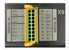
Mount the female FK-MCP 1.5 connector on X9 DIGITAL IN, and connect the wires according to the wiring diagram and the instructions in section 5.2.2 on page 28.
