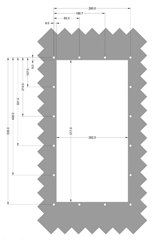
Figure 5 Cabinet cut-out schem for IMD 135
