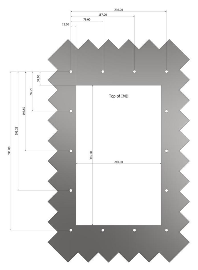
Figure 4 Cabinet cut-out schem for IMD 122
