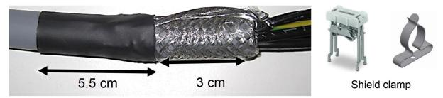
c. IMD 122 A, B, and early C production: Cut 4.5 cm of appropriate shrinkable tube. Shrink the tube around the shield and cable, leaving 4 cm of uncovered shield:
