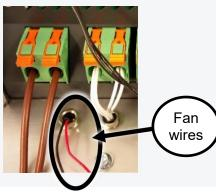
The fan wires are typically (check the wiring diagram) connected directly to DIGITAL OUT connector (X8). The location of the fan wires is indicated in the picture on the left.
