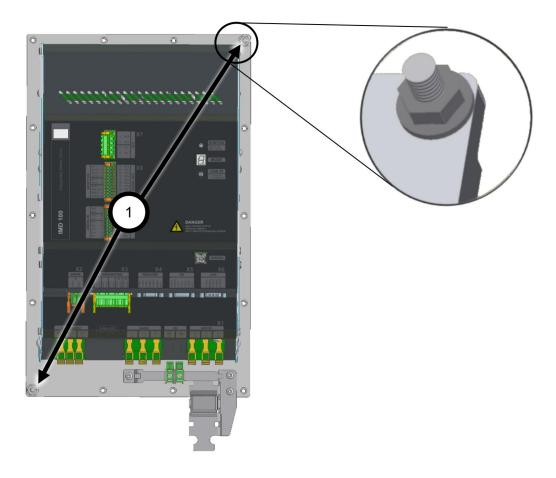
3. Mount all screws around the heat sink (pos. 1) with M6x30 mm screws. Tighten all screws and nuts:
