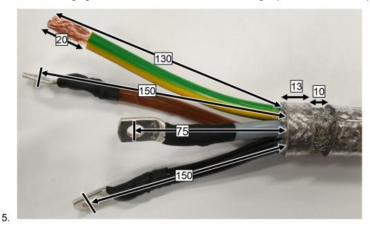
6. The motor cable is now ready for connections.
