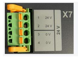
Mount the female FK-MCP 2.5 connector on X7 24 V, and connect the wires according to the wiring diagram and the instructions in section 5.2.2 on page 28.
